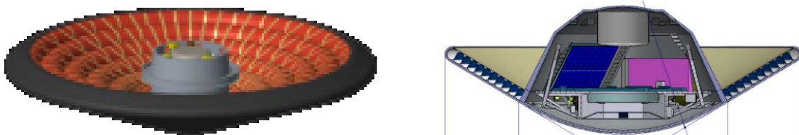
Figure 11-1. HIAD concept for a NASA technology demonstration mission from LEO (left) and an IAD design for a robotic-scale Mars lander from Vorticity Ltd. (right).
